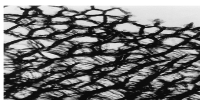
Electron micrograph of nano-structured porous silicon
